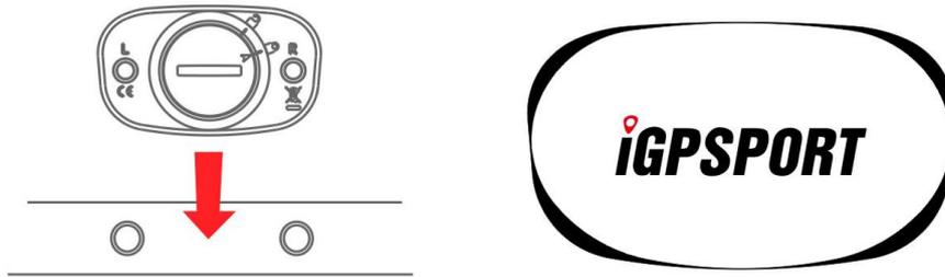
**3.3. Adjust the strap length to fit your chest tightly and comfortably, make sure the wet electrode area touch firmly with your skin(make sure HR40' s left side and right side should be the same as your left hand and right hand).**
